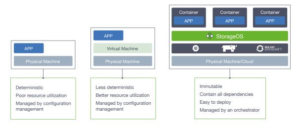
To run applications which require persist storage within containers, we require a layer which can provide persistent disk storage to those containers, independent of the lifecycle of the containers themselves.
