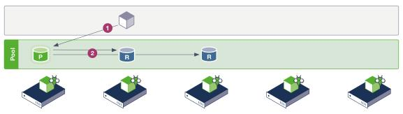
3/4. All acks need to be received by the primary and the write needs to be acknowledged to the application.
