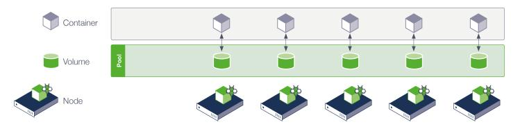
StorageOS features are all enabled/disabled by applying labels to volumes. Labels can be passed to StorageOS via PersistentVolumeClaims (PVCs) or can be applied to volumes using the StorageOS CLI or GUI.
