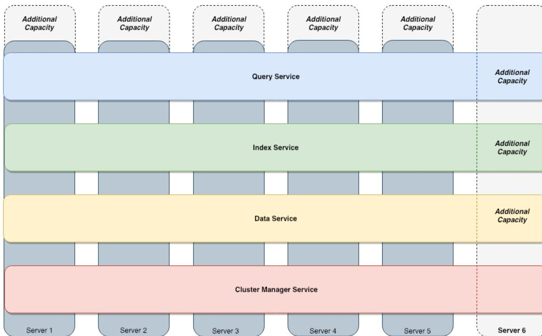
**Figure 3.1.2.1** The homogeneous scaling model of Couchbase Server
