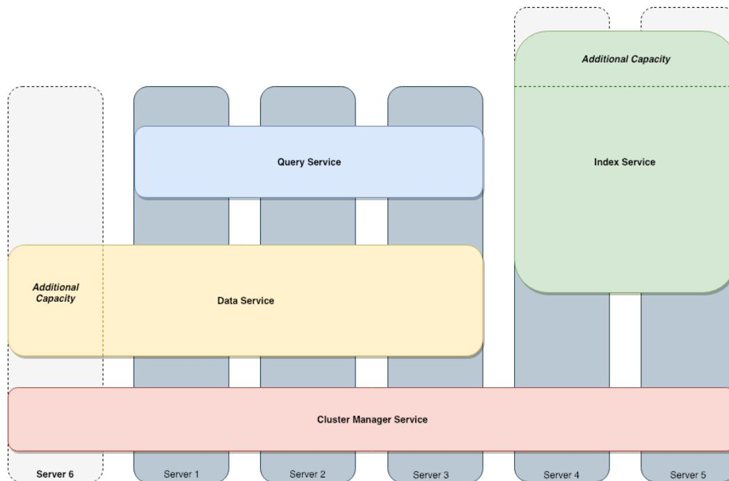
**Figure 3.1.2.2** The independent scaling model of Couchbase Server
