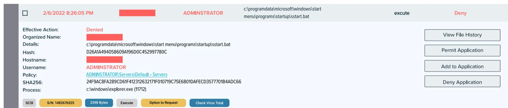
*Figure 2.* An attempted exploit of the Exchange vulnerability that was blocked by blocking a batch file from executing.
