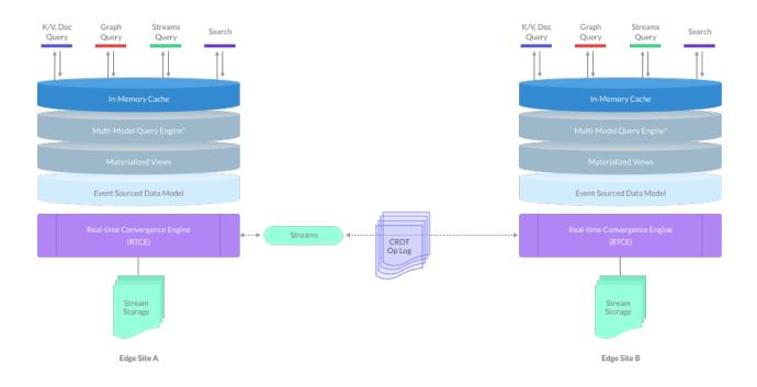
Incoming CRDT ops are processed by our Real Time convergence engine (RICE) to update materialized views in real-time and also stored in event source storage (aka *storage layer*). These views form the *data model layer* providing a common abstraction to support polyglot data model patterns i.e., key-value, doc, graphs, search & streams.
